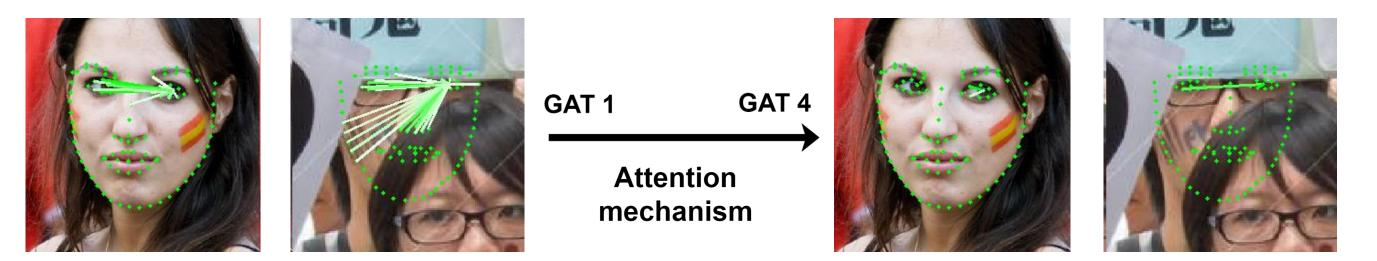
Occlusion images show how the attention mechanism relies on visible ulletlandmarks.
