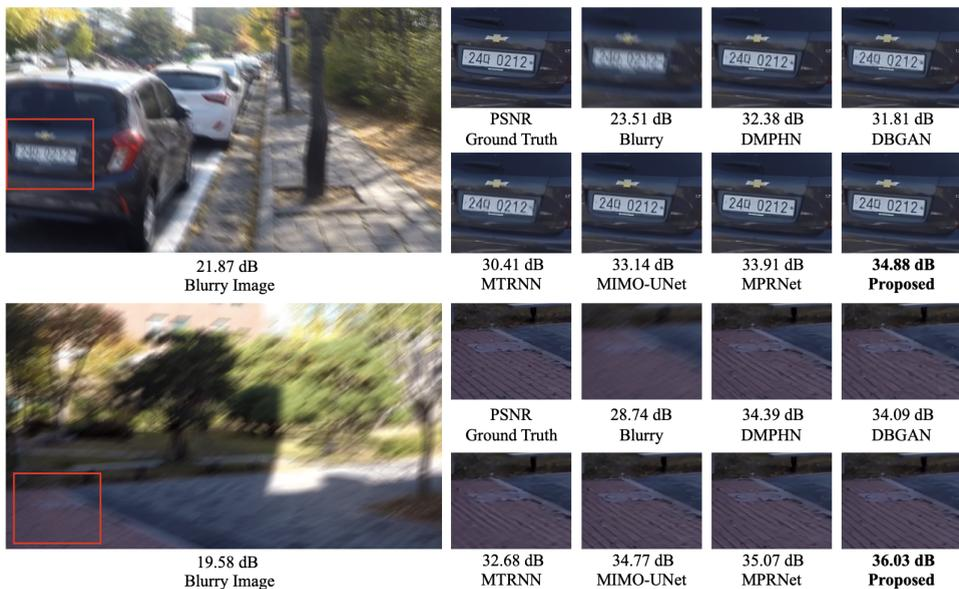
Figure 4: Qualitative comparisons among state-of-the-art method and our proposed SGENet on the GoPro test dataset.
