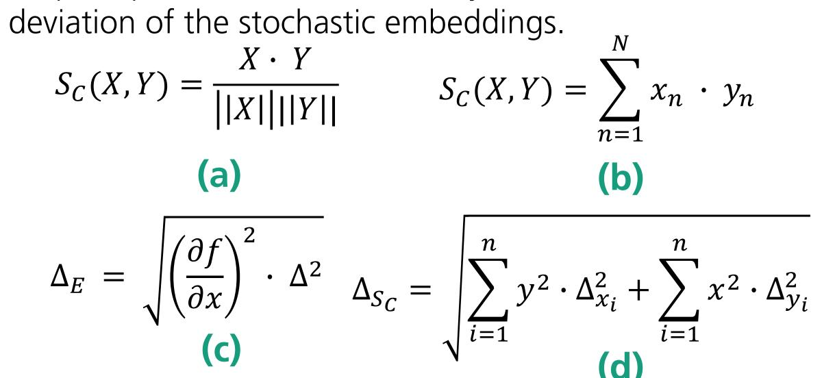
**Uncertainty Estimation of the Comparison Score:** the cosine similarity (a) simplifies to (b) when normalized. The formula of propagation of uncertainty [2] (c) applied to (b) leads to (d), which allows the calculation of the comparison score uncertainty.
