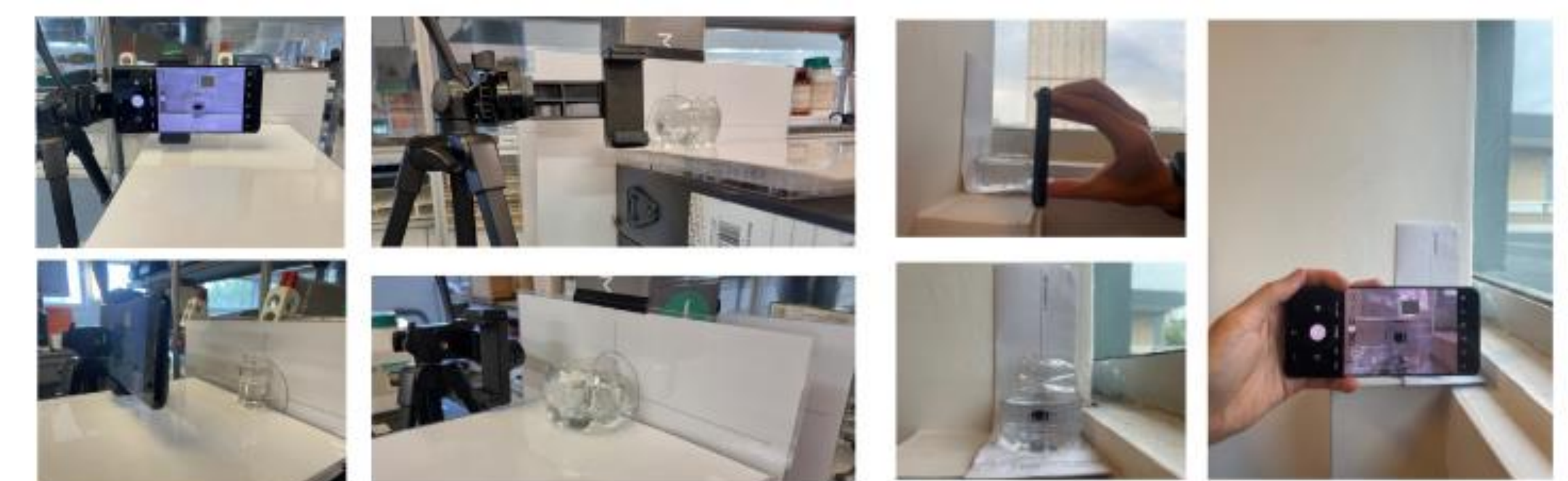
Three dataset collection set-ups. Left: glass container, tripod and indoors. Middle: plastic bottle, tripod and indoors. Right: window, handheld smartphone and plastic bottle.
