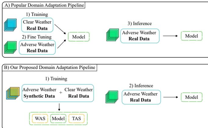
Figure 1: **Existing domain adaptation vs. our proposed pipeline.** Unlike other approaches, our pipeline utilizes synthetic data, Weather-Aware-Supervisor (WAS), and Time-Aware-Supervisor (TAS) to handle standard-to-adverse domain adaptation. Leveraging our synthetic-aware training procedure, we train our weather and daytime-nighttime aware architecture, simultaneously, on synthetic adverse weather and real normal weather data.
