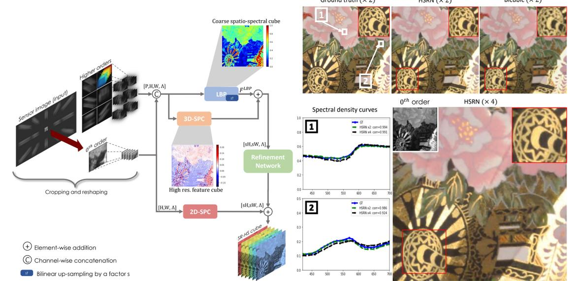
HSRN reconstructs coarse spatio-spectral cubes via LBP which are then added to a high resolution residual generated by 3D-SPC and are further fine-tuned via a dedicated CNN.
