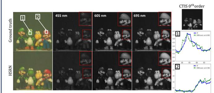
Reconstructed sample with  $\times 2$  the resolution of the  $0^{th}$  diffraction order:  $278 \times 278 \times 25$ .
