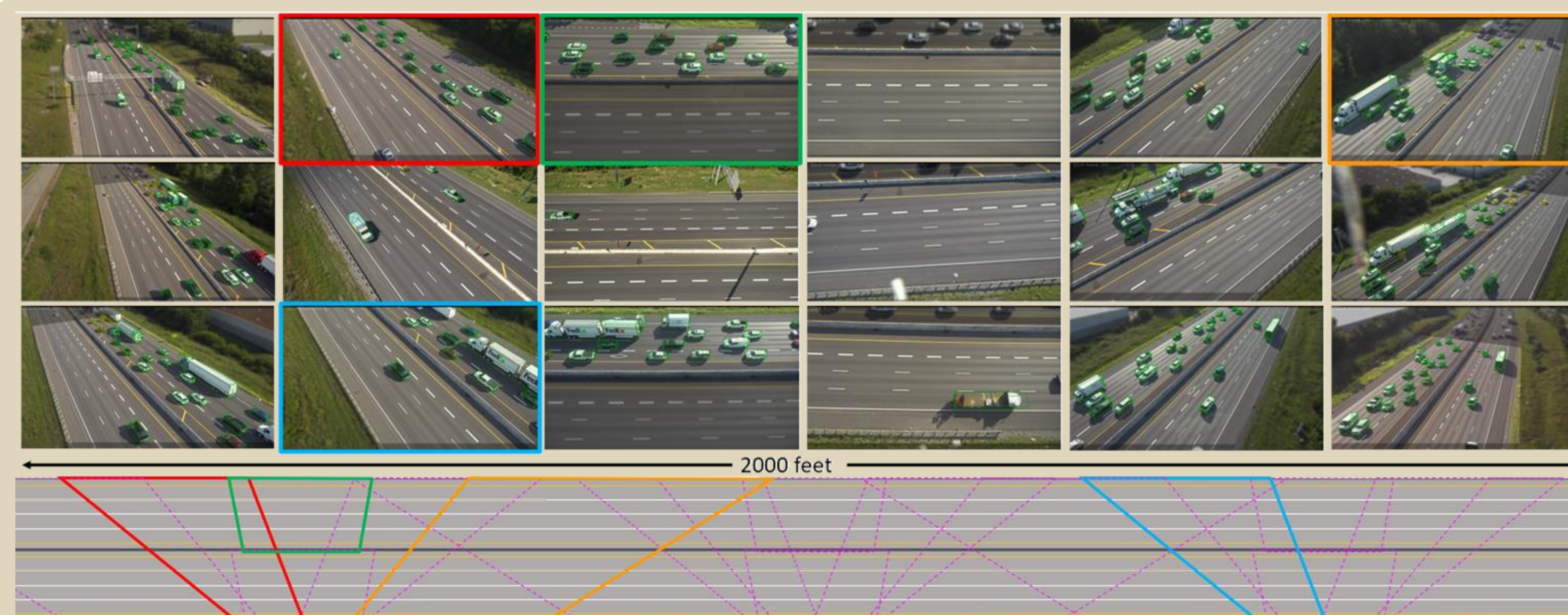
Example frames from each of the 18 cameras used in this work. For selected cameras (red green, blue, orange) the corresponding field of view is shown on an overhead view of the roadway coordinate space. The selected cameras densely cover a 2000-foot portion of the roadway with overlaps.
