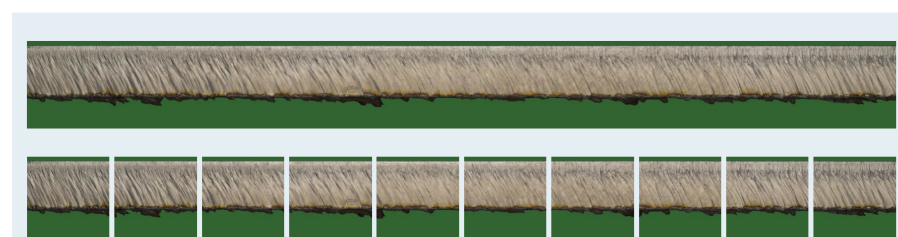
Figure 1: Example of preprocessed images. Using both transmitted and incident illumination allows for simultaneous segmentation, filtering out image regions that are not relevant for quality assessment.
